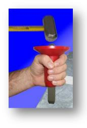
**Safety First** - Durable Technologies' Safety First stamp grip provides improved hand protection and allows the operator to mark with confidence. It is made from a durable, urethane material and features a 4" diameter hand shield that protects the operator's hand during the stamping process. Pocket sizes range from 1/4" to 1" square to accommodate a variety of stamp shank sizes. Ideal for high-volume hand stamping requirements.
