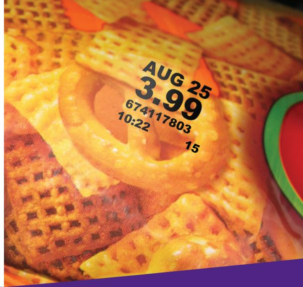
With lower cost and high performance, food and beverage manufacturers are fueling growth of flexible packaging. Variable information like date, price and lot codes are applied to packages via thermal transfer technology. Thermal Transfer Overprinters (TTO) are integrated into vertical and horizontal form, fill and seal equipment, playing a critical role in track and trace and food safety.
